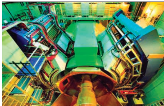
Enormous microscope. The PHENIX detector, one of four that adorn Brookhaven’s RHIC accelerator ring, explores phenomena on the tiniest scales accessible to humans.
